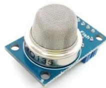
Gambar 2. Sensor Gas MQ-135
