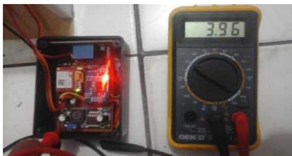
Gambar 11. Pengujian power supply daya GSM Shield SIM 800
