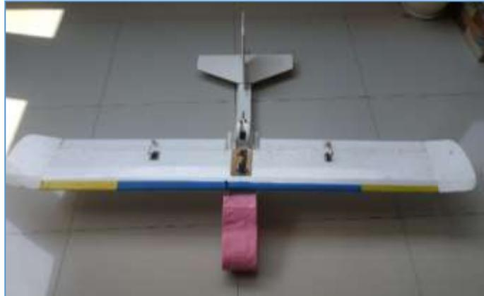
**Gambar 5 Pesawat Fixed Wing FT-Explorer**
